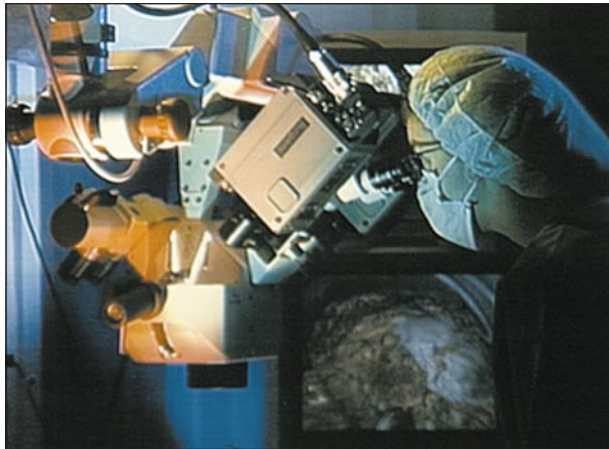
Figure 4. Stereoscopic surgical microscope with 2 independent remote channels for second opinion. (Source: SRU OP 2000 RRK/MDC, Berlin, Germany.)
