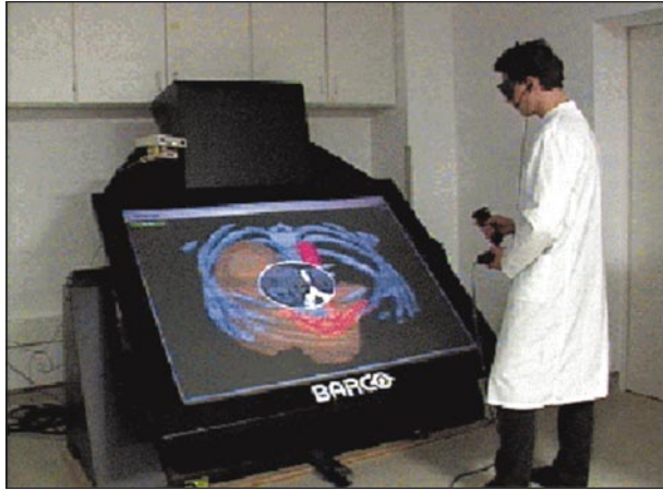
Figure 2. Virtual surgical table for medical simulations with haptic interfaces and voice control. (Source: OP 2000 RRR/MDC, Berlin, Germany and GMD, St Augustin, Germany.)
