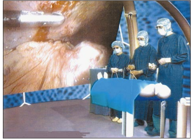
Figure 3. Virtual interactive laparoscopy. A team of surgeons is captured by 2 tracked cameras (from a blue box) and projected into a virtual operating room. Manipulations on the virtual patient are illustrated by projecting videos of former laparoscopic investigations. (Source: OP 2000 RRR/MDC, Berlin, Germany and GMD, St Augustin, Germany.)
