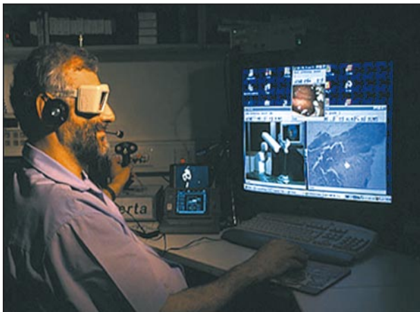
Figure 5. Stereoscopic workstation with interactive telemedical facilities. Three video sources are displayed simultaneously: 3-dimensional room camera, 3-dimensional laparoscope, and biopsy examination. (Source: SRU OP 2000 RRK/MDC, Berlin, Germany.)
